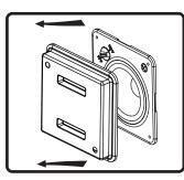
**6.** Remove paint mask unless painting is required. In that case, follow steps 7-10 when painting is complete.
